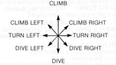
POWER forward is selected by pressing a number key on main keyboard, (or key pad) from **1** (low) through **9** with **0** = maximum thrust. Reverse thrust is achieved by pressing  $\langle$ **SHIFT** $\rangle$  and a number simultaneously. Fine adjustment to the power level is achieved by pressing keypad ' $\rightarrow$ ' key to increase and ' $\leftarrow$ ' key to decrease. For zero forward thrust, which permits hover on certain craft, press  $\langle$ **SPACE BAR** $\rangle$ .
