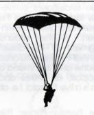
• Parafoil: Not the usual globe-canopy parachute, a parafoil is shaped more like an airplane wing. This shape is difficult to control, but in the hands of an expert it enables the parachutist to glide forward rather than drop straight down. The 'chutist can control the direction of the glide by pulling down on the left or right. This action spills air out one side of the foil, causing it to pivot on the other side and turn in the direction of the pull. Since turning spills air,
