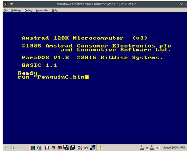
We can also run the game by terminal executing the command `$ cpct_winape PenguinCross.dsk` in the folder where DSK file is located and it automatically write `run"penguinc.bin` and load the game.
